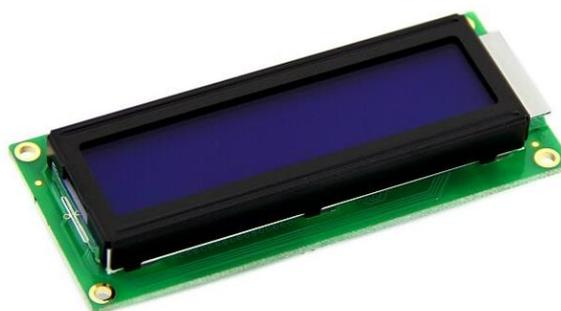
**Gambar 2.8 LCD 16x2 [12]**
