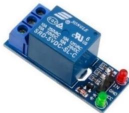
**Gambar 2.7 Relay 1 Channel [8]**
