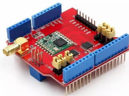
Gambar 3.3 LoRa Shield SX1276/SX1278 [41].
