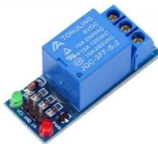
**Gambar 2.9 Relay 1 channel [27]**
