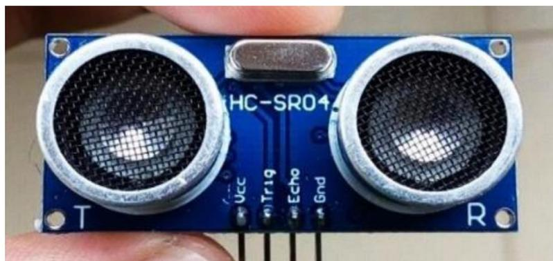
**Gambar 2.3 Sensor ultrasonik [20]**
