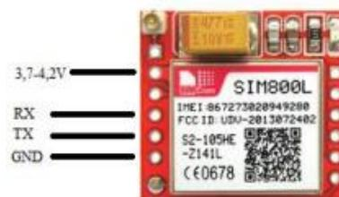
Gambar 2.8 Modul GSM SIM800L [15]
