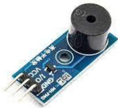
Gambar 2. 7 Modul *Buzzer*
