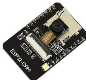
Gambar 2. 5 NodeMCU ESP32 Cam
