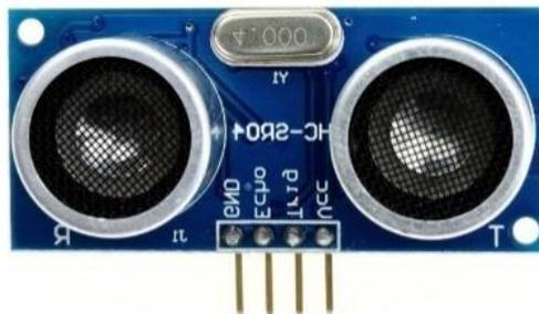
**Gambar 2.5 Sensor Ultrasonik HC-SR04 [23]**
