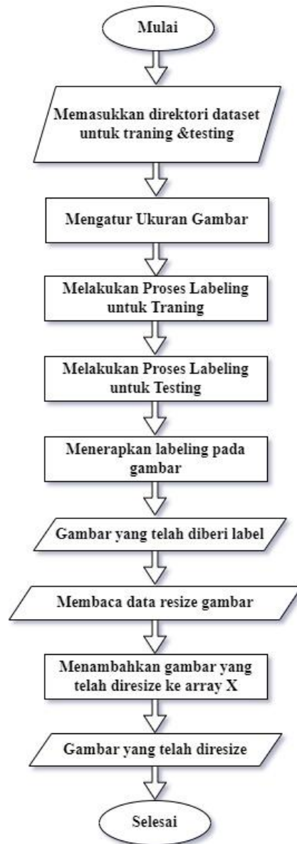
Gambar 3. 3 flowchart Proses Pre-Processing
