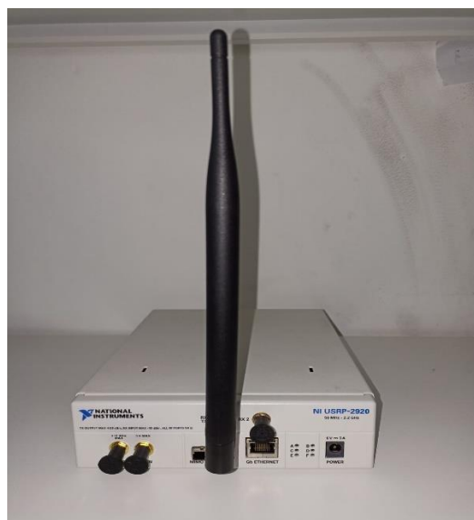
Gambar 2.9 Instalasi Antenna Monopole [21].
