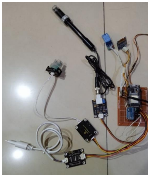
Gambar 3.4 Rancangan sensor TDS, Turbidity, pH dan LYNX-32
