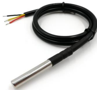
Gambar 2.8 Sensor Suhu DS18B20 [29]
