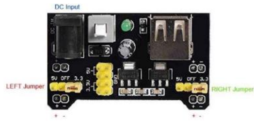
Gambar 2. 7 Breadboard Power Supply MB102
