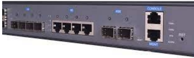
Gambar 2.4 Optical Line Terminal [2].
