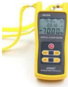
Gambar 2. 10 Optical Power Meter (OPM) [8].
