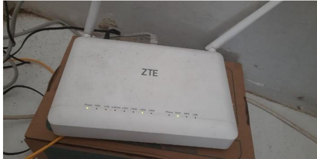
Gambar 2.6 Optical Network Terminal [2].
