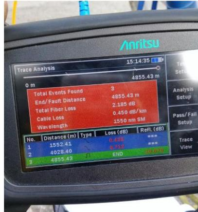
Gambar 2.8 *Optical Time Domain Reflectometer* [12].
