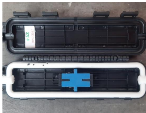
Gambar 2.13 OTP ( Optical Termination Premisses )
