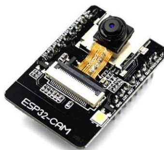
Gambar 2. 4 Tampilan Board ESP32-CAM
