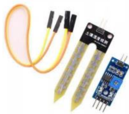
Gambar 2. 3 Soil Moisture Sensor (YL-69) [13]
