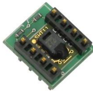
Gambar 2.9 Sensor suhu SHT11[10]
