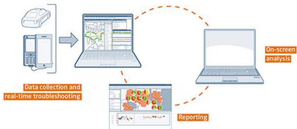
Gambar 2.8 Konsep dasar Drive Test [11]
