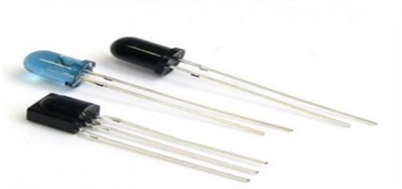
Gambar 2.11 LED Infra Merah [11]
